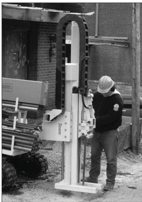
TOP LEFT: Examining a soil sample. TOP RIGHT: Checking an abandoned drum. ABOVE: Setting up a geoprobe to take soil samples. Photos by DCA
